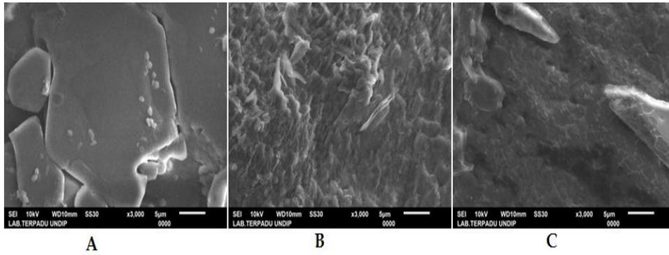
Figure 2. Morphology of (a) Urea fertilizer (b) UC (c) UZC
